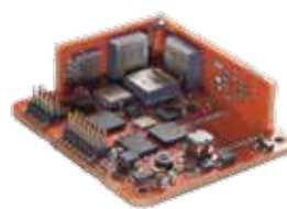
OEM: 37x33x12 mm, 11g, 24-pins header
