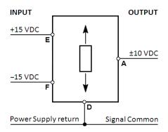
A through F: Connector pin assignments
