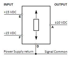
A through F: Connector pin assignments
