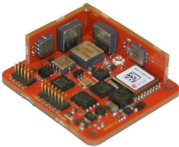
MTi OEM: 37x33x12 mm, 11g, 16-pins header
