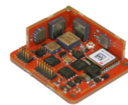
MTi-G-710 OEM: 37x33x12 mm, 11g, 16-pins header
