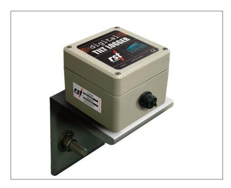
The Digital Tilt Logger is a low cost, battery-powered data logger and tilt meter in a single compact unit. It measures tilt in either one or two perpendicular axes in the plane of the base. The unit is intended to be permanently installed to provide long-term observation with maximum resolution and sensitivity, and is conveniently designed for manual monitoring or remote data acquisition.
