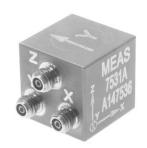
The Model 7531A is an adhesively mounted triaxial charge mode accelerometer with an operating temperature range to +260°C. The accelerometer is designed for high frequency vibration and shock measurements and offers a wide bandwidth to >10kHz with a nominal charge output of 1.8pC/g. The model 7531A incorporates stable high temperature piezo-ceramic crystals in annular shear mode
