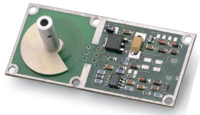
calibration and automated testing assures a nonlinearity error of less than ±0.5% of full scale.
