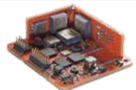
OEM: 37x33x12 mm, 11g, 24-pins header
