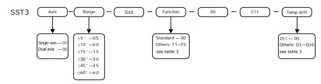
For example, if order a dual-axis USB inclinometer, with range  $\pm 15^{\circ}$ , the accuracy at room temperature is  $\pm 0.02^{\circ}$ , same the range of  $-20 \sim 60^{\circ}$ , USB output, 2m shield cable, anti-vibration module, the model should be SST302-15-G10-F5 -00-C11-D3 (2m, enclosed referred disk (dynamic library, source code and instruction)
