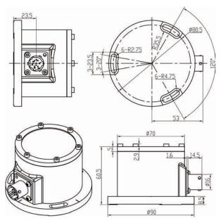
Picture 2 Housing with MIL class connector
