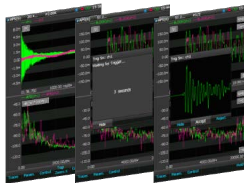
Figure 5: Acquisition Modes 'Free-Run', 'Auto-Trigger', and 'Manual Trigger'
