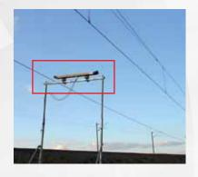
The small size of the OVHWizard allows a wide range of application in contact wire position detection. The OVHWizard can be used on:
