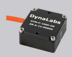
These capacitive accelerometers are reliable and long-term stable. They have DC response. The advantage of these sensors is their outstanding temperature stability, their lightweight and they are low cost sensors. These sensors have reliable aluminum housing with IP68 protection class. Dynalabs 1000DE series accelerometers provide an outstanding noise performance from 25 to 170  $\mu$ g/  $\sqrt{Hz}$ . These accelerometers provide a wide frequency range (±3dB) from 1,500 Hz to 3,000 Hz.
