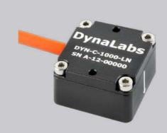
These capacitive accelerometers are reliable and long-term stable. They have DC response. The advantage of these sensors is their outstanding temperature stability and their lightweight. These sensors have reliable aluminum housing with IP68 protection class. Dynalabs 1000LN series accelerometers provide an outstanding noise performance from 9 to 680  $\mu$ g/ $\forall$ Hz. These accelerometers provide a wide frequency range ( $\pm$ 5%) from 700 Hz to 2,900 Hz.
