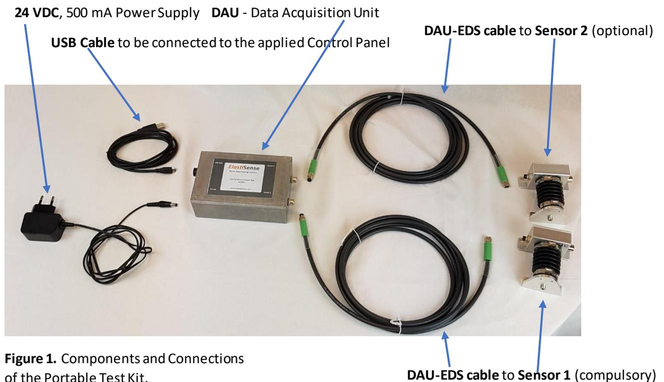
**Figure 1.** Components and Connections of the Portable Test Kit.
