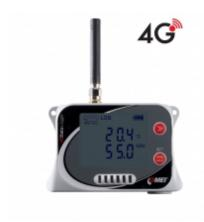
GSM datalogger is designed to record temperature and humidity from built-in sensors. In case of exceeded set limits, SMS and JSON messages can be sent via 4G data connection. Measured values can be sent to the internet storage <a href="COMET Cloud">COMET Cloud</a>, which is a complete monitoring, alarm and analysis system.
